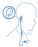
When you're not using your headset, keep the earpiece in the holder. Press the earpiece firmly into the holder so it stays in place. The headset switches off automatically.
