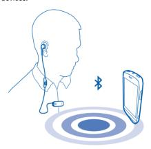
This device is compliant with Bluetooth Specification 2.1 + EDR supporting the following profiles: headset profile (1.1), handsfree profile (1.5). Check with the manufacturers of other devices to determine their compatibility with this device.
