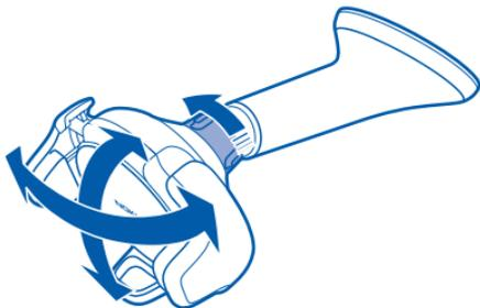
**Tip:** Holder not turning easily? To loosen the tightening nut, turn it clockwise.
