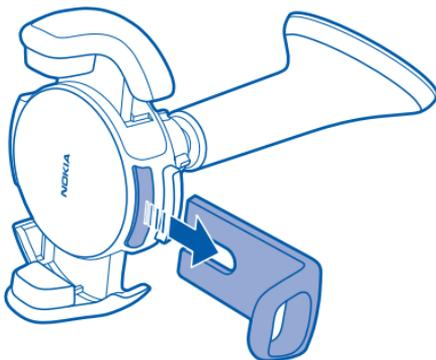
3 To widen the clamps, lift and hold the clamp release lever.
