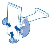
5 Push the clamps together, until the phone is firmly in place.
