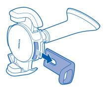
3 To widen the clamps, lift and hold the clamp release lever.
