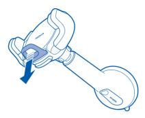
4 Place your phone in the holder, and adjust the bottom support, until the phone is at a height where it is secure.
