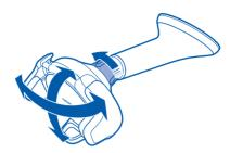
Tip: Holder not turning easily? To loosen the tightening nut, turn it clockwise.
