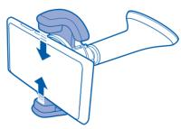
5 Push the clamps together, until the phone is firmly in place.
