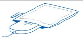
Open the fastening on the short end of the pillow, and pull the charging plate out.
