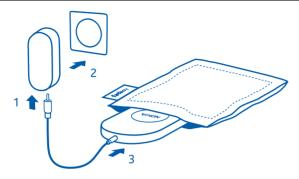
Use the charging plate only with the supplied power supply.
