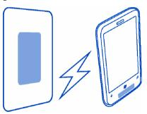
Qi works using magnetic induction, and is currently designed for devices that use 5 watts of power or less, such as mobile phones. Qi chargers and devices use the same frequency, so as long as their active areas are touching, all Qi products are compatible, regardless of manufacturer or brand. For more details, see the user guides of both devices.
