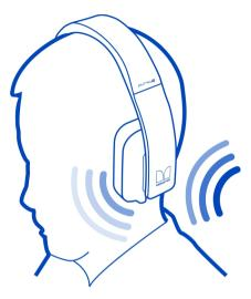
When you put your headset on, the earpiece proximity sensors switch ANC on automatically. When you take the headset off, ANC switches off.
