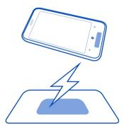
Qi works using magnetic induction, and is currently designed for devices that use 5 watts of power or less, such as mobile phones. Qi chargers and devices use the same
