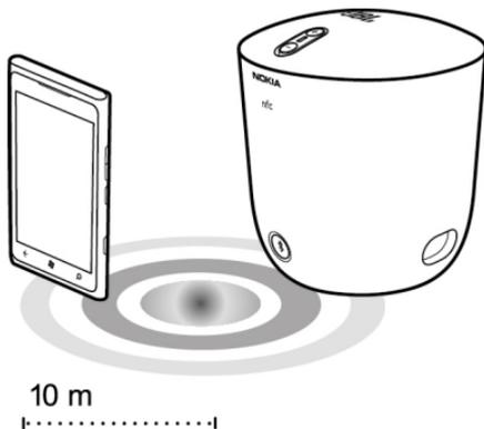
This device is compliant with Bluetooth Specification 2.1 + EDR supporting the following profiles: A2DP and AVRCP. Check with the manufacturers of other devices to determine their compatibility with this device.
