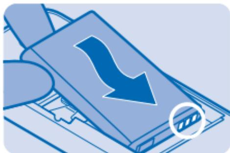
**4.** Line up the battery contacts, and push the battery in.
