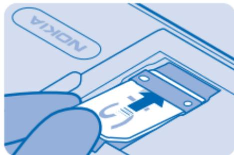
**3.** Slide the SIM under the holder with the contact area face down.
