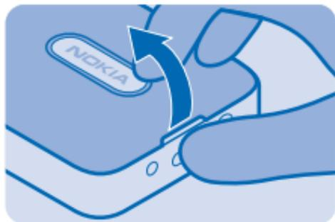
**1.** Switch the phone off, and remove the back cover.
