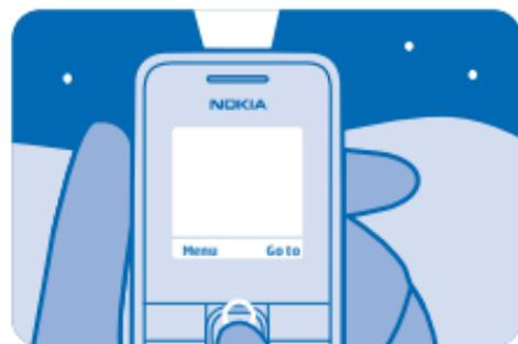
6. To use the flashlight, press the scroll key up twice. To switch off, press up once. Do not shine the light in anyone's eyes.
