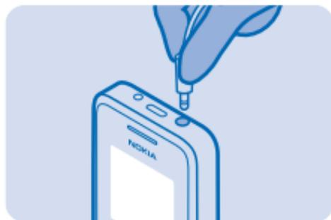
1. Connect a headset, and select **Menu > Radio**. The headset cable works as the radio antenna.
