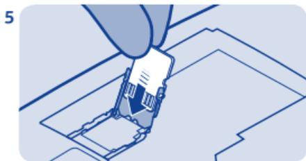
Put a compatible memory card in with the contact area face down.
