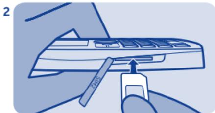
Put the SIM in with the contact area face up.
