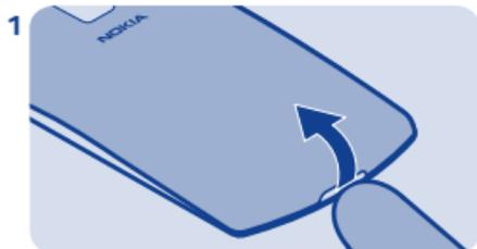
Switch the phone off, and remove the back cover.
