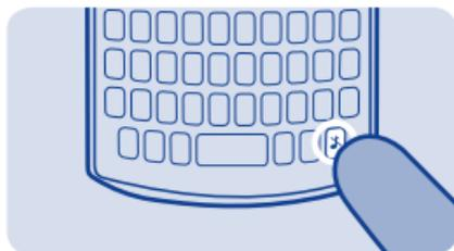
**Tip:** To switch between the silent and normal profile, press and hold
