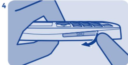
To remove the card, open the **SIM2** SIM cover.
