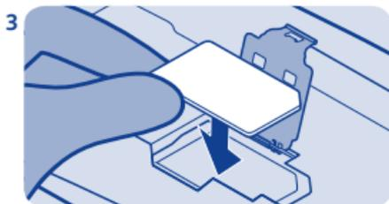
Lift the SIM card holder, and place the SIM in the holder with the contact area face down. See
