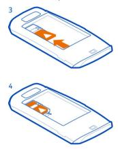
4 Line up the battery contacts, push the battery in (5), then replace the back cover (6).
