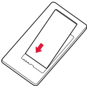
7. Press the bottom edge of the back cover against the bottom edge of your phone, and snap the cover into place. Don't press the keys while attaching the cover.
