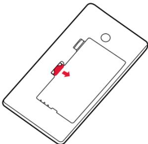
5. To remove the memory card, slide it out from the slot.
