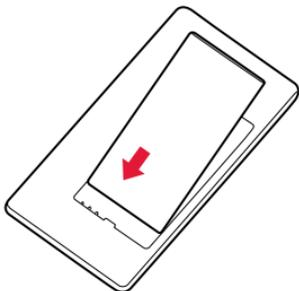
6. Press the bottom edge of the back cover against the bottom edge of your phone.
